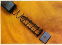
Magazine from Model 38/42 was prone to failure, and with no time to redesign spring in WWII, problem was solved by insertion of 10-round horseshoe-shaped spacer inside magazine body.
